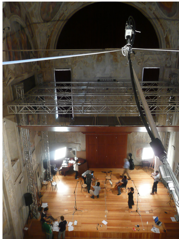
Figure 2: set up of the string quartet experiments at our research centre: the picture shows other video-cameras for movement analysis, lighting systems for motion tracking, and the setup of physiological on-body sensors to musicians (in collaboration with Ben Knapp (SARC, University of Belfast)).
