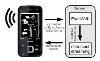
**Figure 2**: Mobile Orchestra Explorer architecture when audio rendering is sent back to the mobile phone: user moves in the orchestra space by tilting the mobile phone; user position is sent to Max/MSP for audio generation and audio is sent back in real-time to the user mobile phone.
