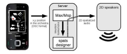
**Figure 1**: Mobile Orchestra Explorer architecture when using the 2D spatializer speaker: the user moves in the orchestra space by tilting the mobile phone; user position is sent to Max/MSP for audio generation and audio is produced by the 2D spatializer speaker.
