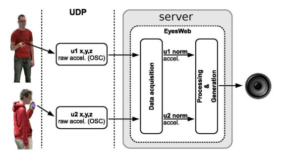
**Figure 4**: Sync'n'Move architecture: users move their mobiles, the raw accelerations are detected and analyzed. A multitrack audio content is generated according to the phase synchronization degree reached by the users.
