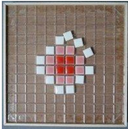
Figure 8: Plates for Lining Up Color Tiles
