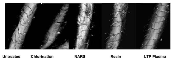
Figure 2: Photographs of the surfaces of the wool fibers without and with treated physicochemical processing.
