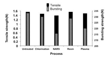
Figure 5: Tensile and bursting strength of the fabrics subjected to anti-pilling processing.
